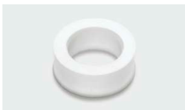
51 161 102 | Silicone rubber sealing ring with vulcanized-on PTFE washers for GL14 caps and sensors with outer Ø 8 mm
